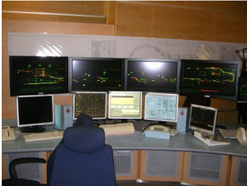
Figure 15: Rail traffic management (RTM) controller's workstation at the RCC on the French side
