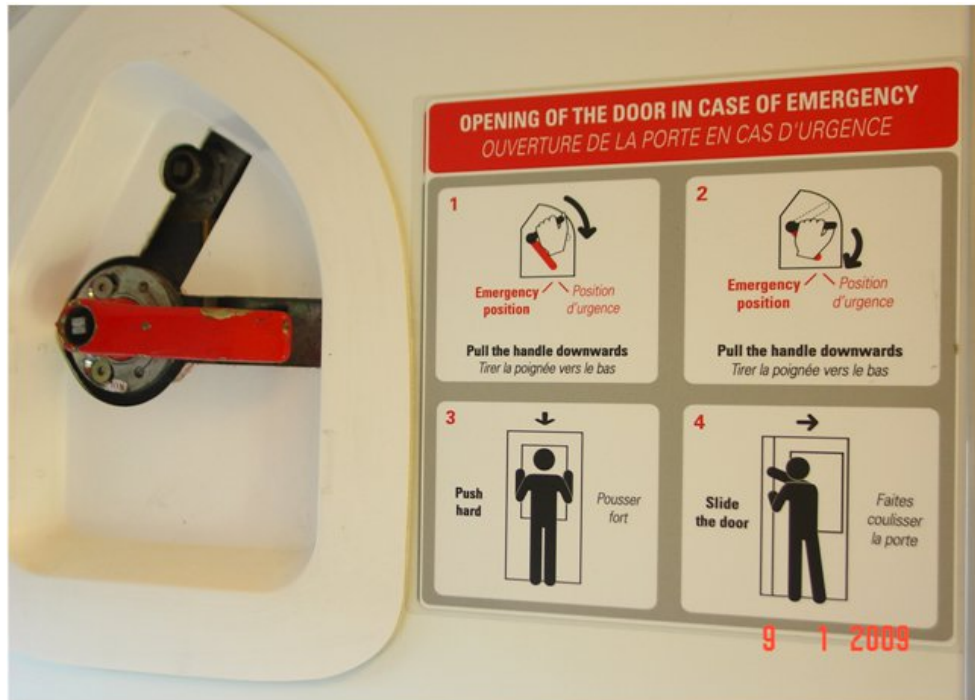
Figure 21: Amenity coach, manual door-release device, operated by a handle
