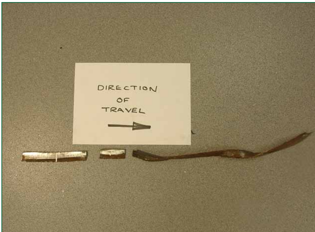
Figure 5: The failed section of the keep
