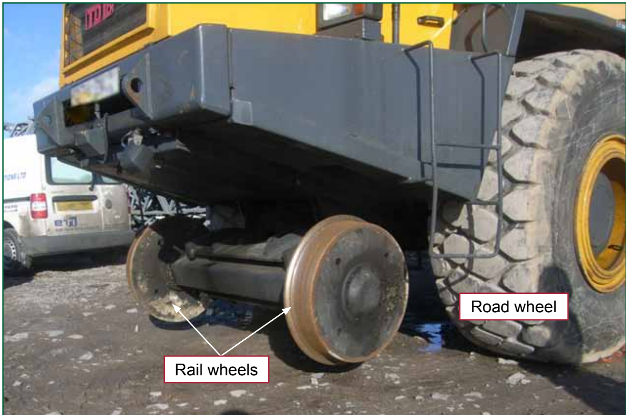
Figure 12: TD-18 RRV rail gear at the front of the machine
