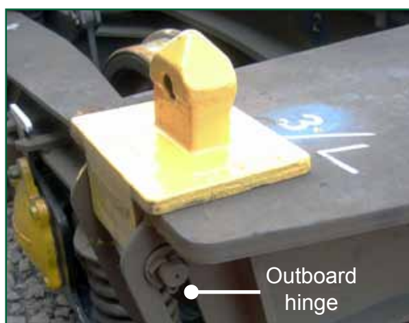
Figure 13: Example of fold-down UIC spigot with outboard hinge (FEA-A wagon)
