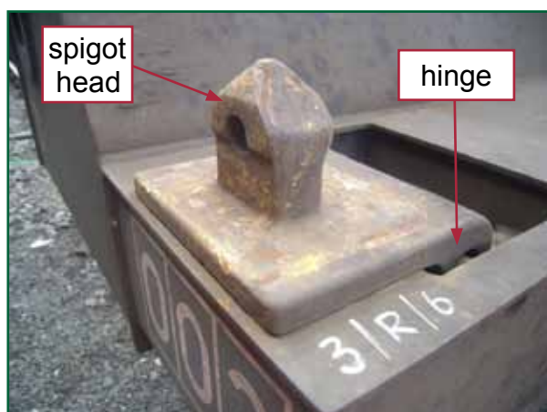
Figure 6: Fold-down spigot with inboard hinge, as fitted to FEA-B wagons, deployed (left), stowed (right)
