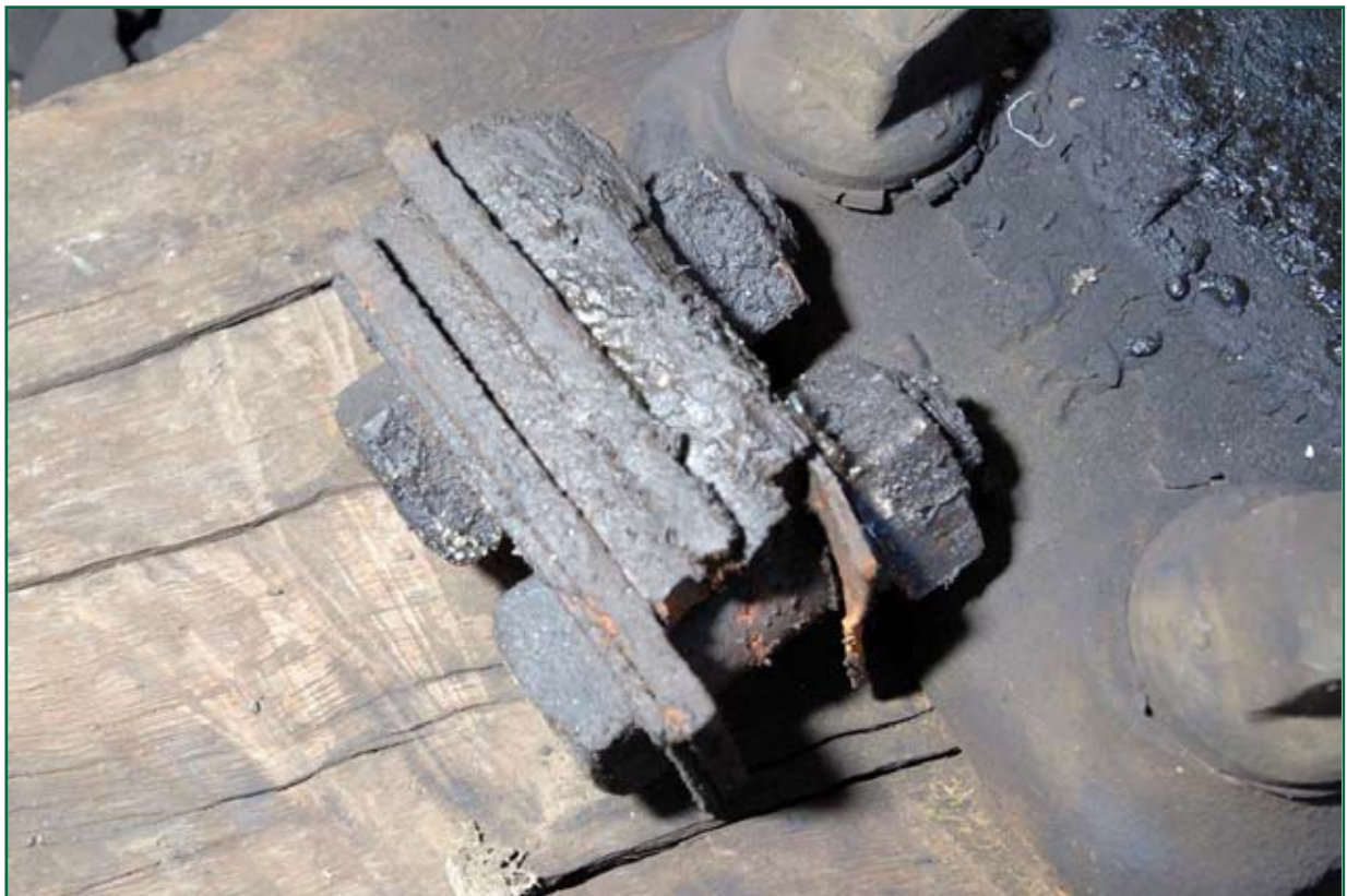
Figure 15: Swan neck from third stretcher bar lying on bearer (24 February 2007)
