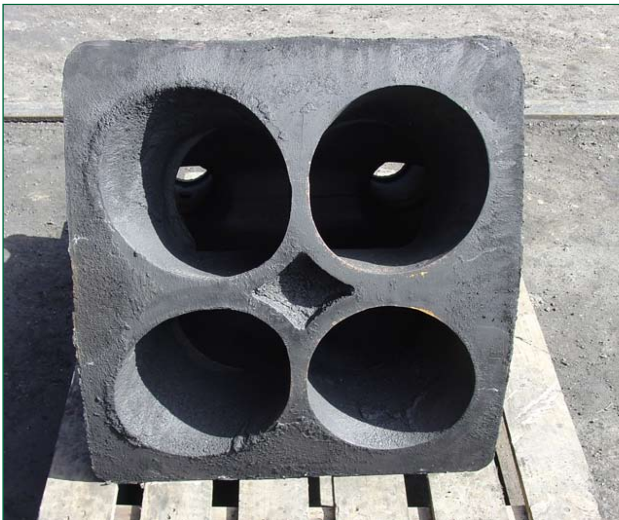
Figure 9: The underside of the blastpipe base
