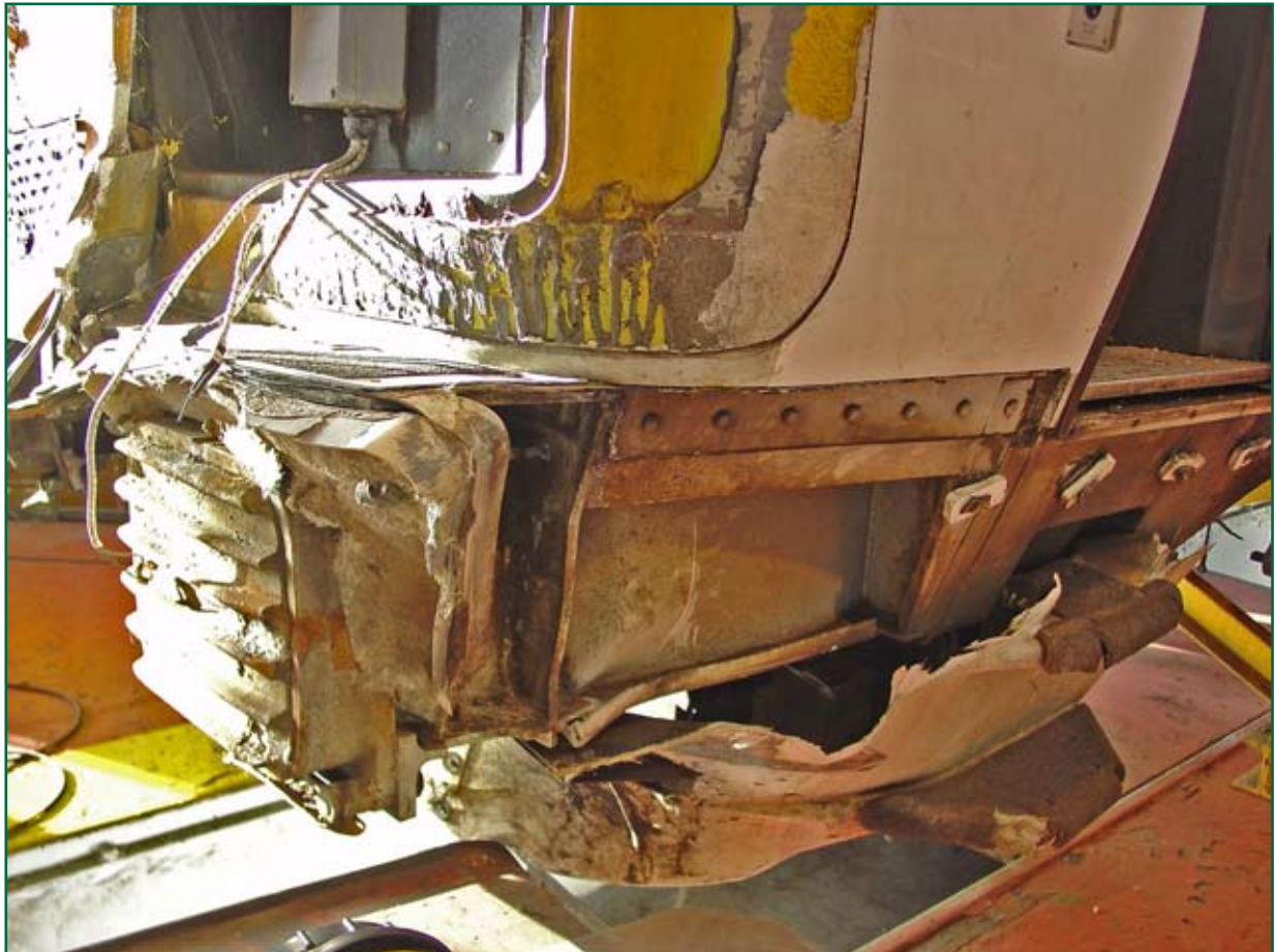
Figure 13: Damage at left side of train
