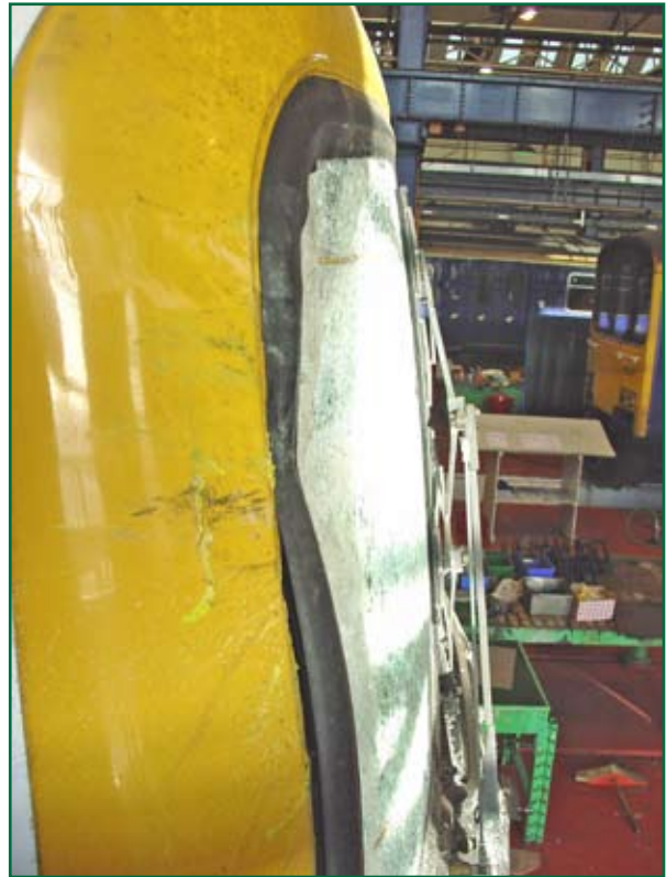
Figure 10: Front of train showing impact marks from tractor cab
