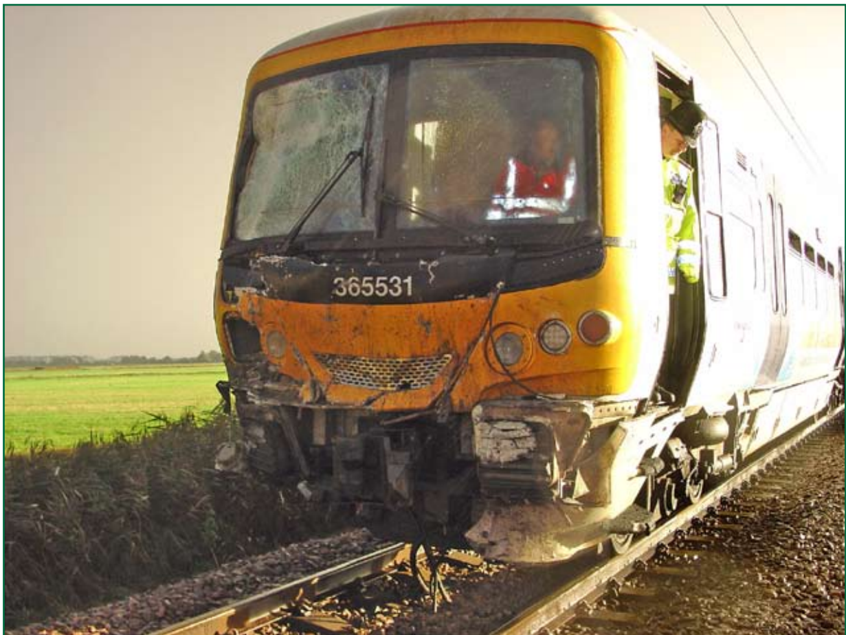
Figure 11: Damage to front of train
